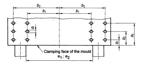
Figure 1: Position and size of mounting holes
